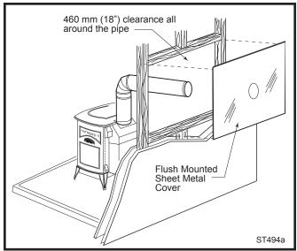
Fig. 8 An approved wall pass-through.
